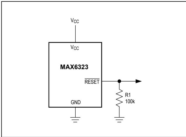
Figure 6.  $\overline{\text{RESET}}$  Valid to  $V_{CC} = \text{Ground}$  Circuit
