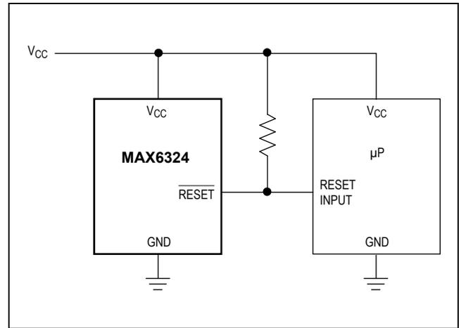
Figure 7. Interfacing to µPs with Bidirectional Reset Pins
