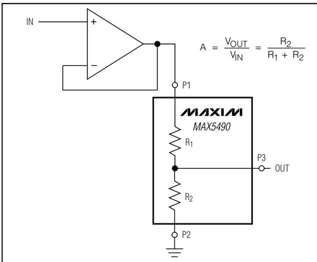
Figure 3. Buffered Attenuator
