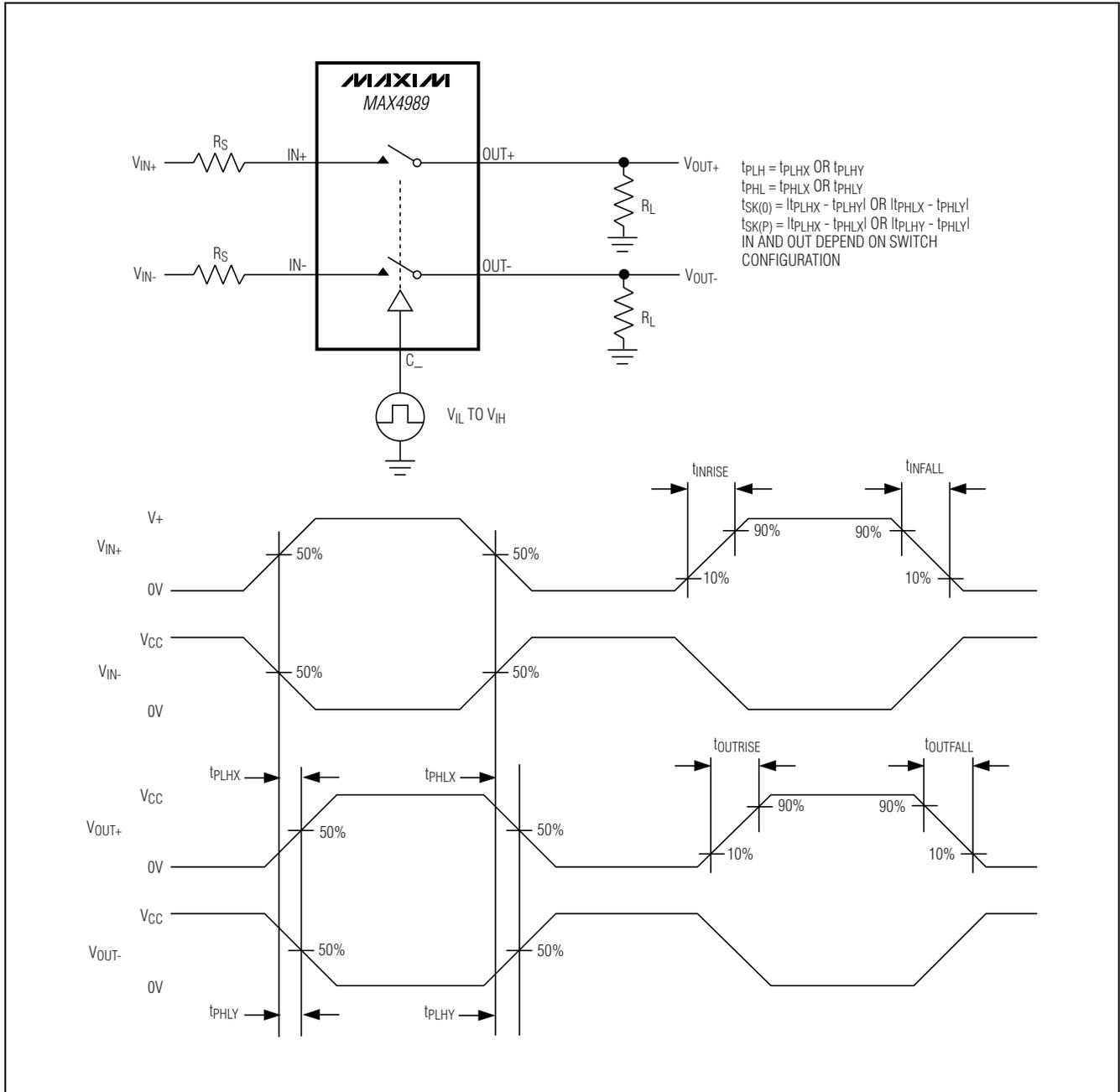
Figure 3. Output Signal Skew, Rise/Fall Time, Propagation Delay
