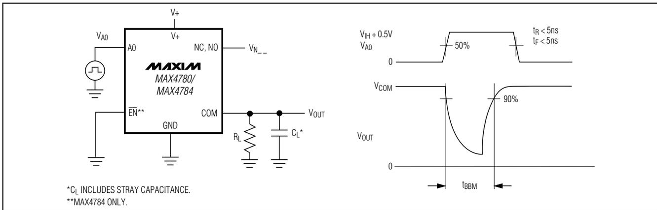
Figure 2. Break-Before-Make Interval
