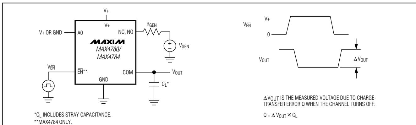
Figure 3. Charge Injection
