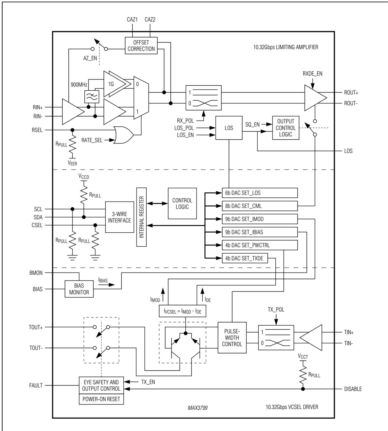
Figure 2. Functional Diagram
