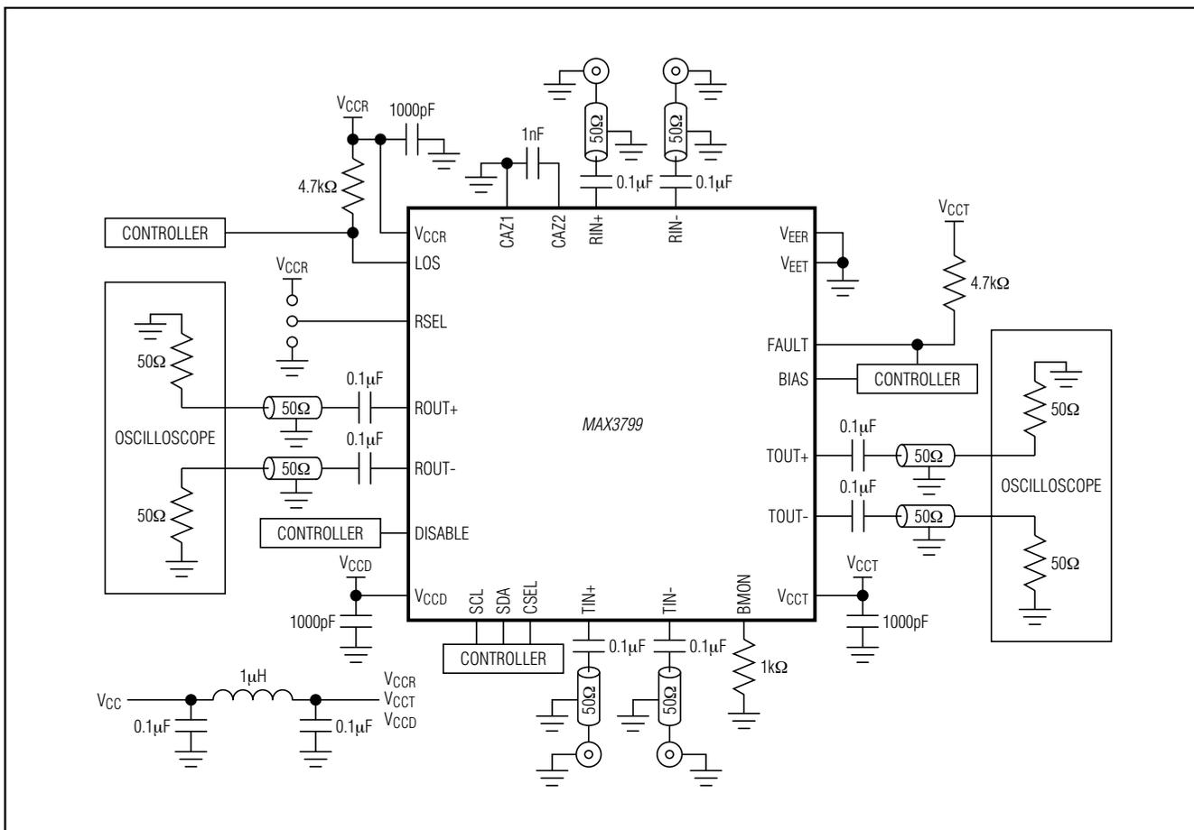
Figure 1. Test Circuit for VCSEL Driver Characterization
