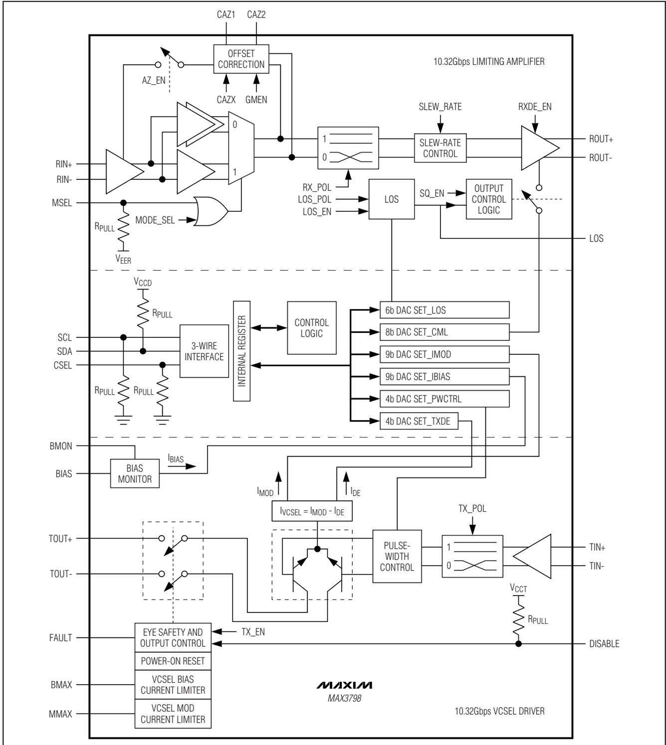
Figure 2. Functional Diagram
