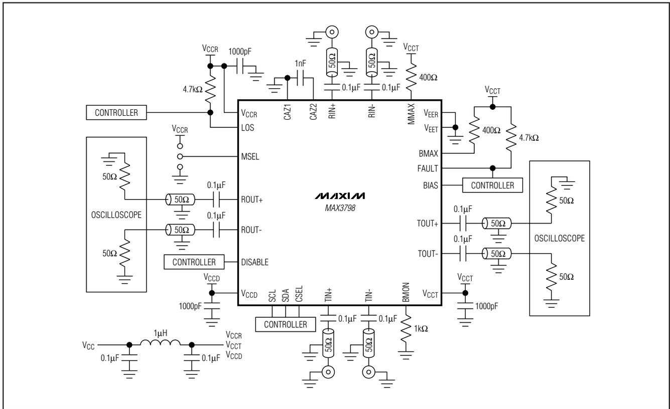
Figure 1. Test Circuit for VCSEL Driver Characterization
