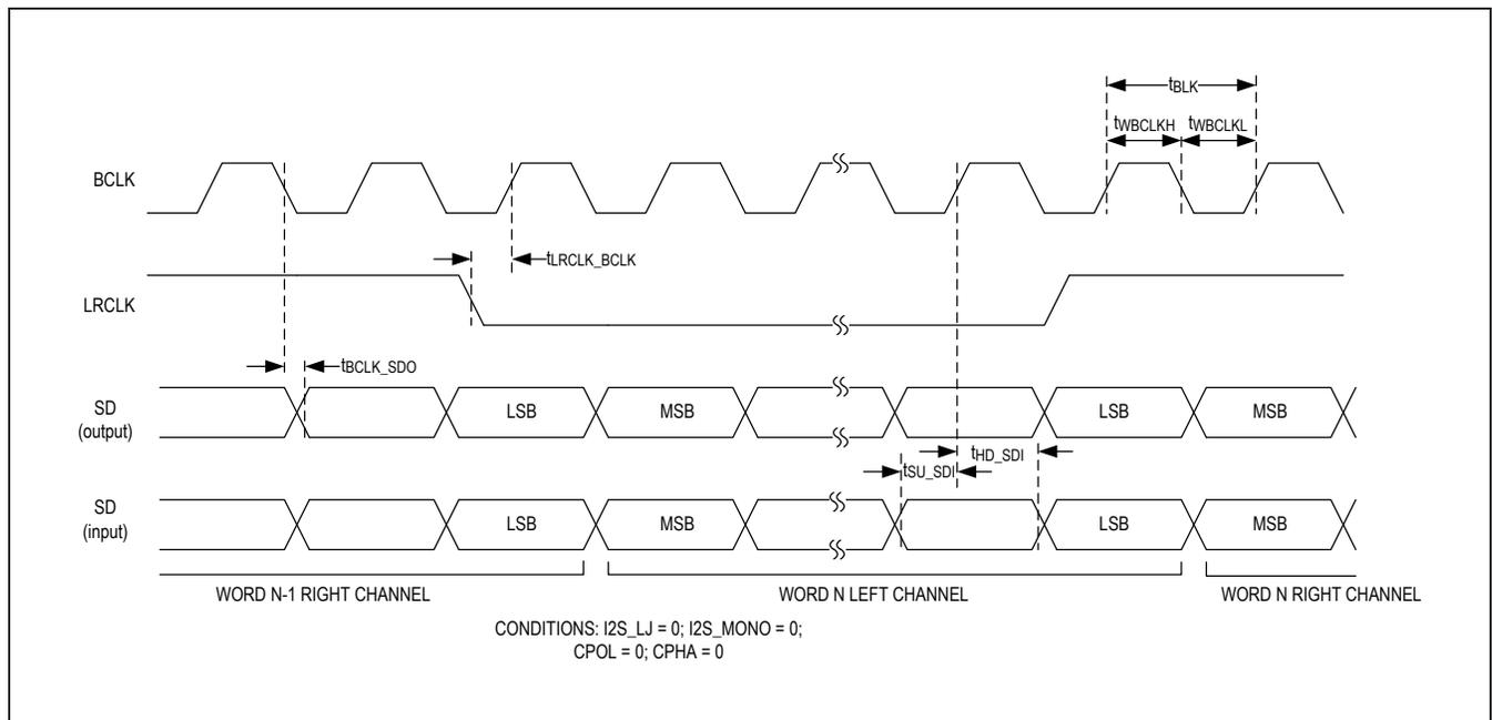
Figure 5. I<sup>2</sup>S Timing Diagram
