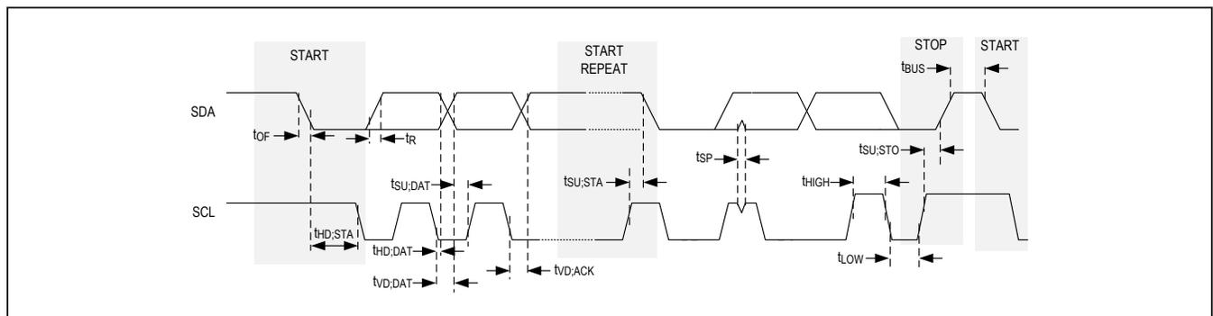
Figure 4. I<sup>2</sup>C Timing Diagram
