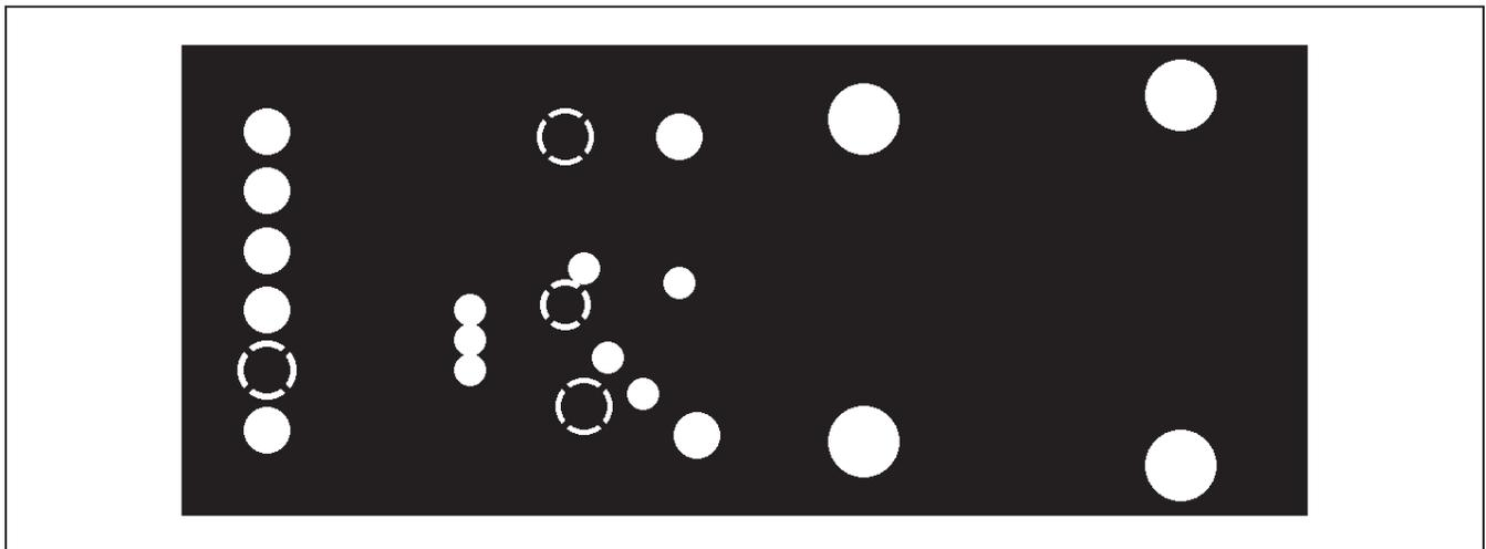
Figure 4. MAX31855PMB1 Peripheral Module PCB Layout—Inner Layer 1 (Ground)
