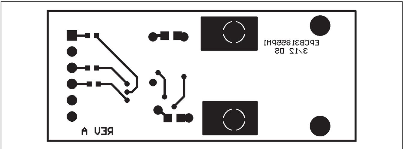
Figure 6. MAX31855PMB1 Peripheral Module PCB Layout—Solder Side
