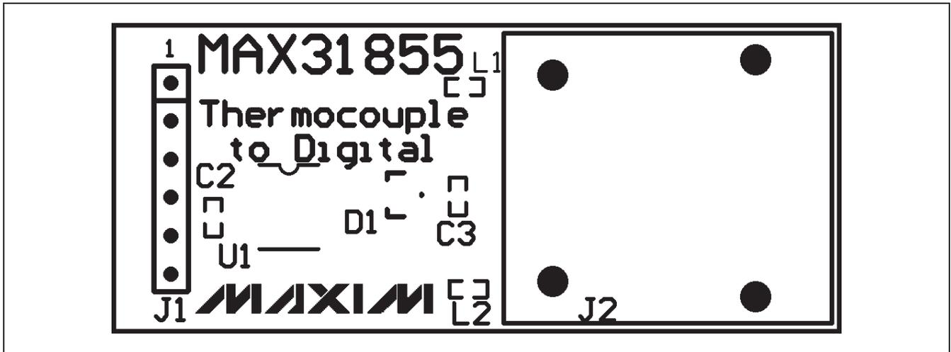
Figure 2. MAX31855PMB1 Peripheral Module Component Placement Guide—Component Side
