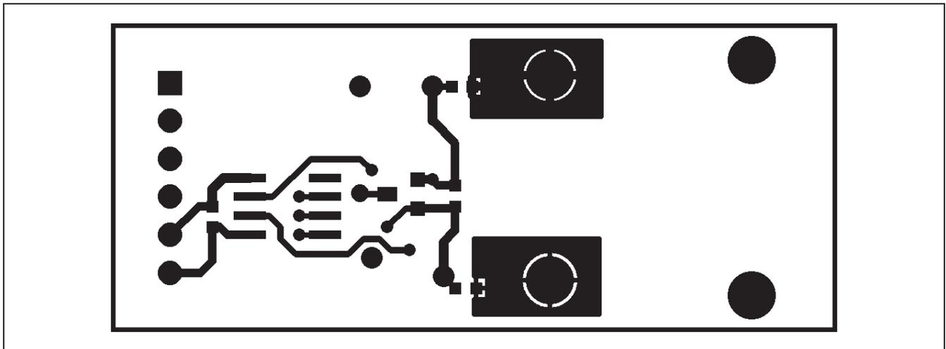
Figure 3. MAX31855PMB1 Peripheral Module PCB Layout—Component Side
