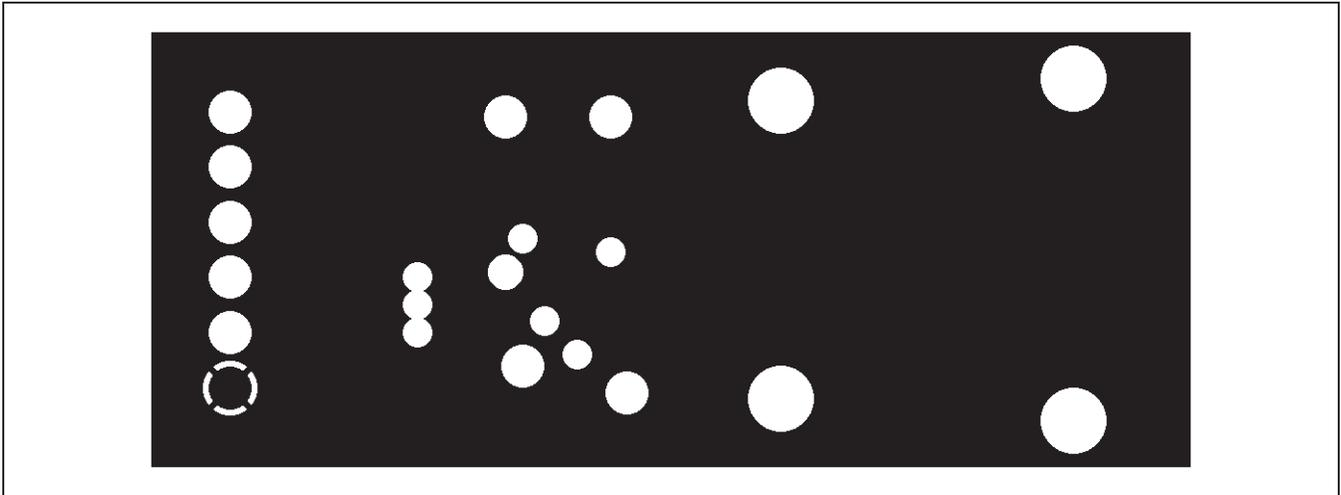
Figure 5. MAX31855PMB1 Peripheral Module PCB Layout—Inner Layer 2 (Power)
