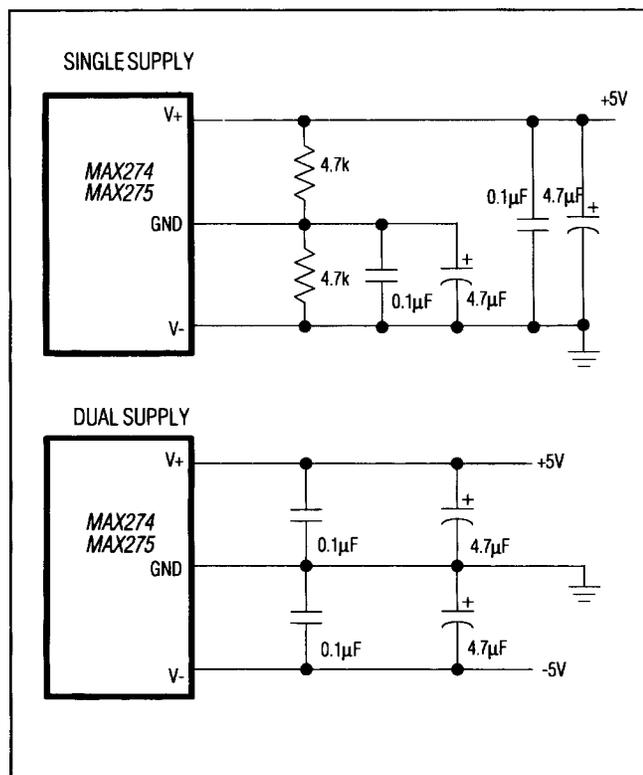
Figure 9. Power-Supply Configurations
