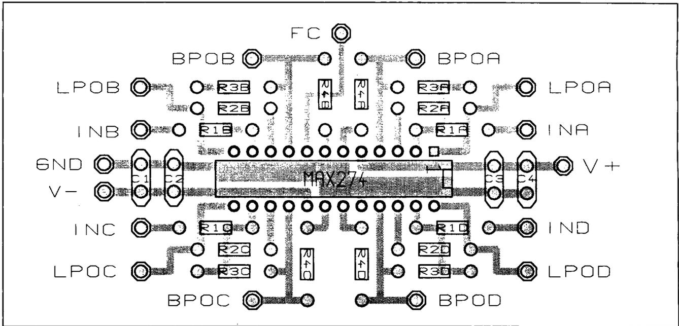
Figure 7a. MAX274 Suggested PC-Board Layout for DIP
