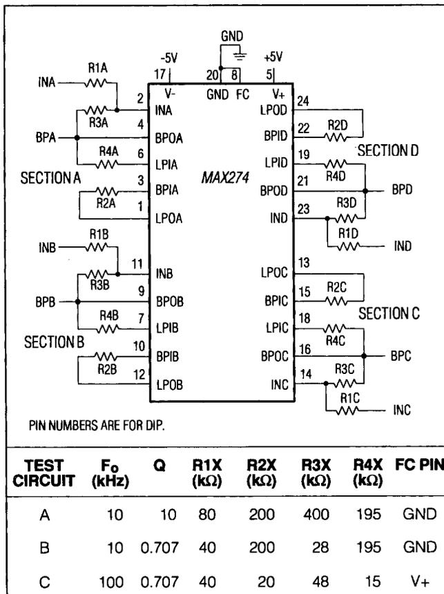
Figure 1a. MAX274 Connection Diagram and Test Circuit
