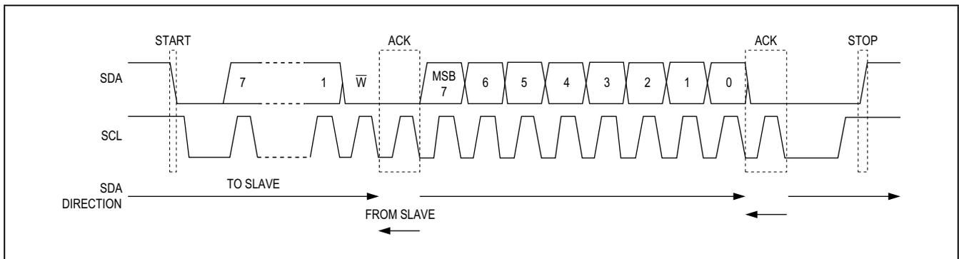
Figure 22. Write Transaction
