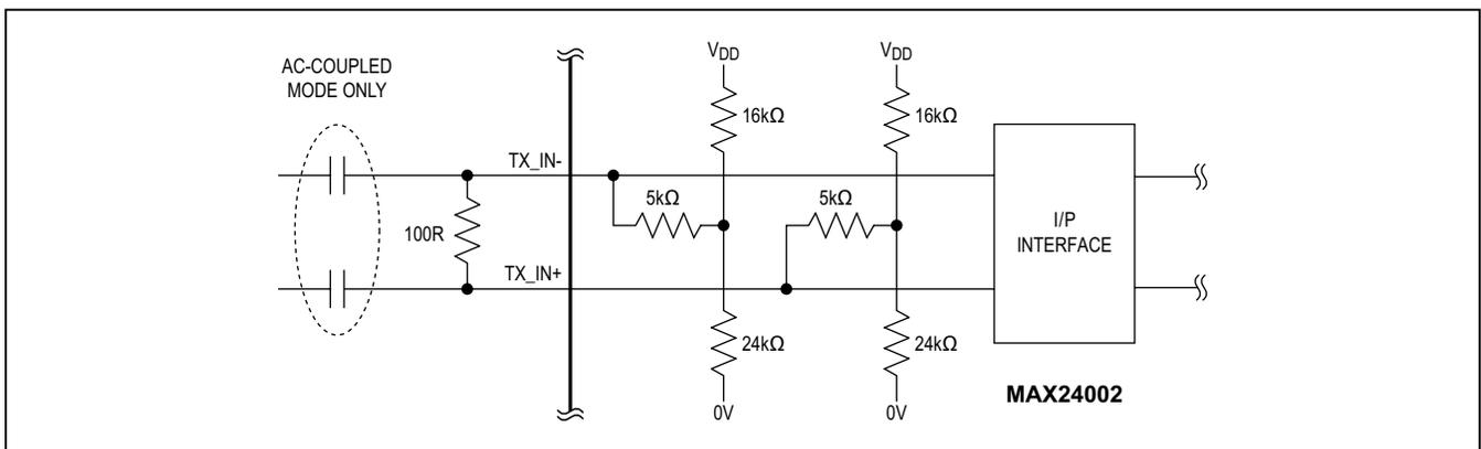
Figure 5. TX\_IN Input Termination and Signal Conditioning
