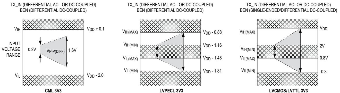
Typical I/O ranges for TX\_IN are shown
