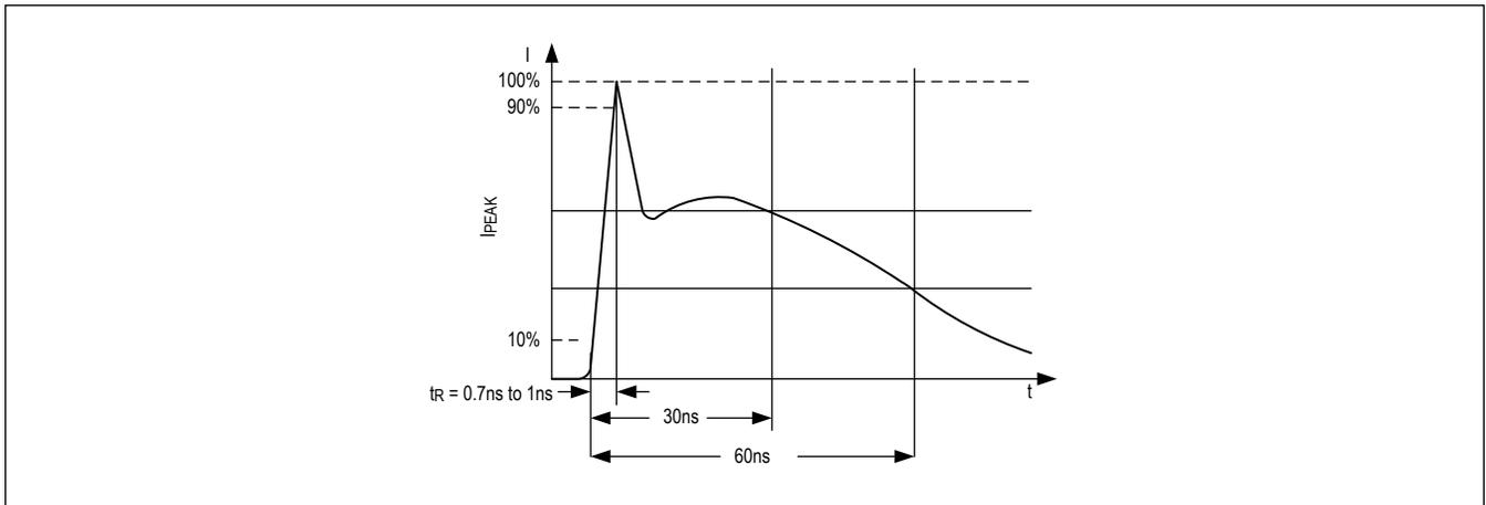
Figure 13. IEC 61000-4-2 ESD Generator Current Waveform
