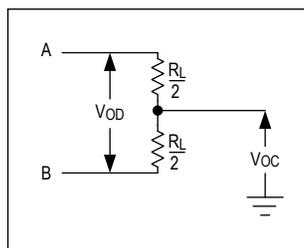
Figure 1. Driver DC Test Load
