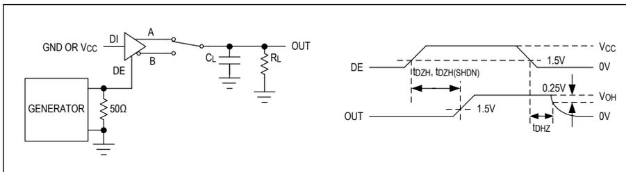
Figure 4. Driver Enable and Disable Times ( $t_{DZH}$ ,  $t_{DZH}$ )
