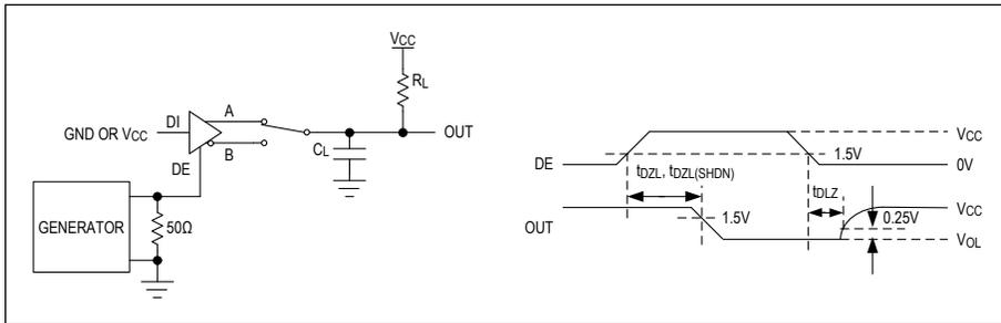
Figure 5. Driver Enable and Disable Times ( $t_{DZL}$ ,  $t_{DLZ}$ )
