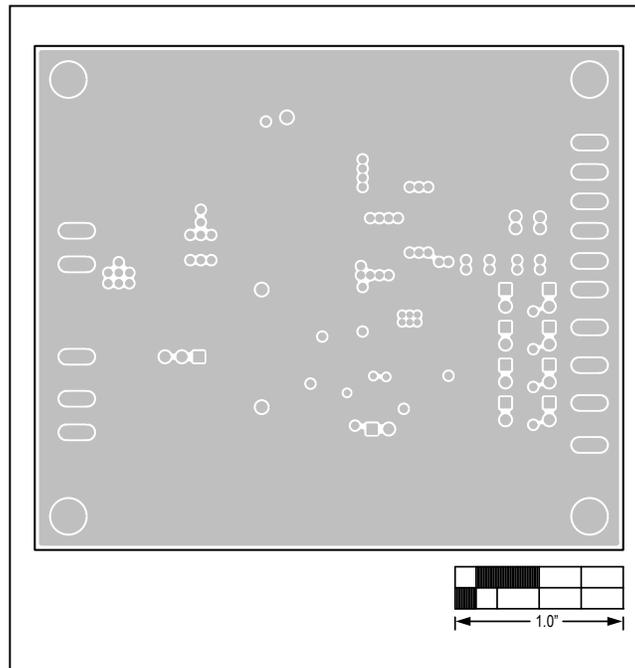
Figure 4. MAX16813 EV Kit PCB Layout—SGND Layer 2
