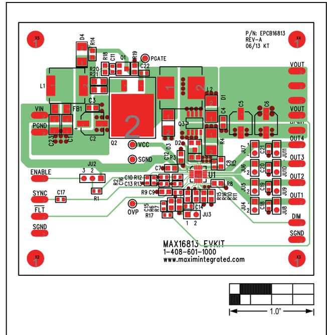
Figure 3. MAX16813 EV Kit PCB Layout—Component Side
