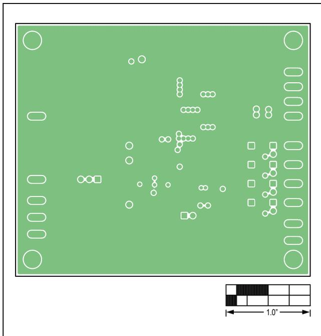
Figure 5. MAX16813 EV Kit PCB Layout—PGND Layer 3
