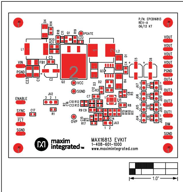
Figure 2. MAX16813 EV Kit Component Placement Guide—Component Side
