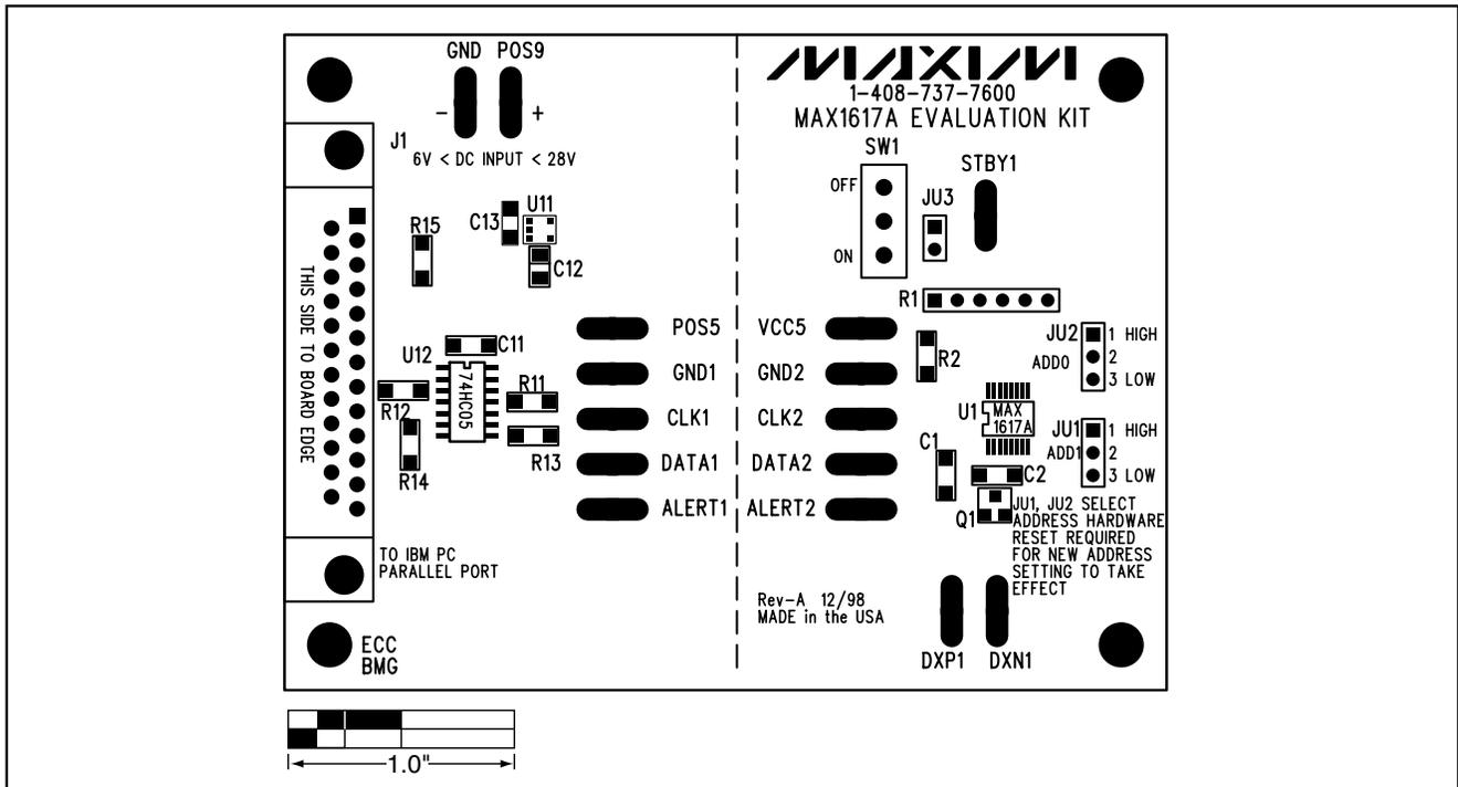
Figure 2. MAX1617A EV Kit Component Placement Guide
