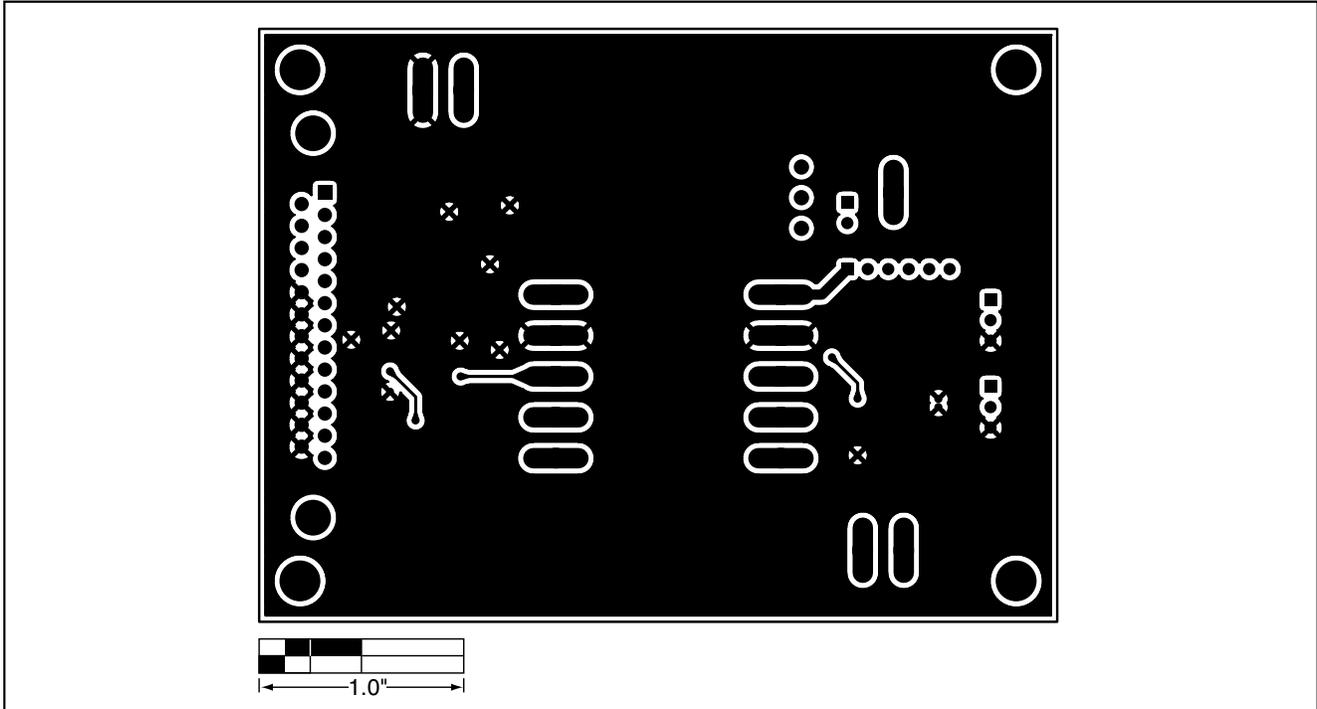
Figure 4. MAX1617A EV Kit PC Board Layout—Solder Side
