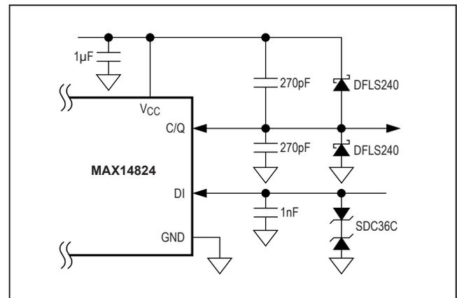
Figure 11. MAX14824 Operating Circuit with TVS Protection
