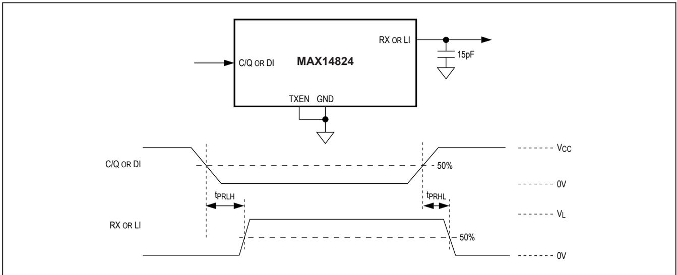
Figure 4. Receiver Polarity and Timing
