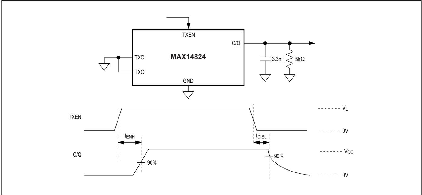
Figure 3. Driver Enable High and Disable Low Timing
