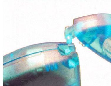
**\*Note:** The data contact faces down and away from the embossed ‘i’. Once the iButton is inserted in the enclosure, snap the end cap over it. The end cap is removed by depressing the release tab with a paper clip, swinging it fully open, and sliding out the hinge.
