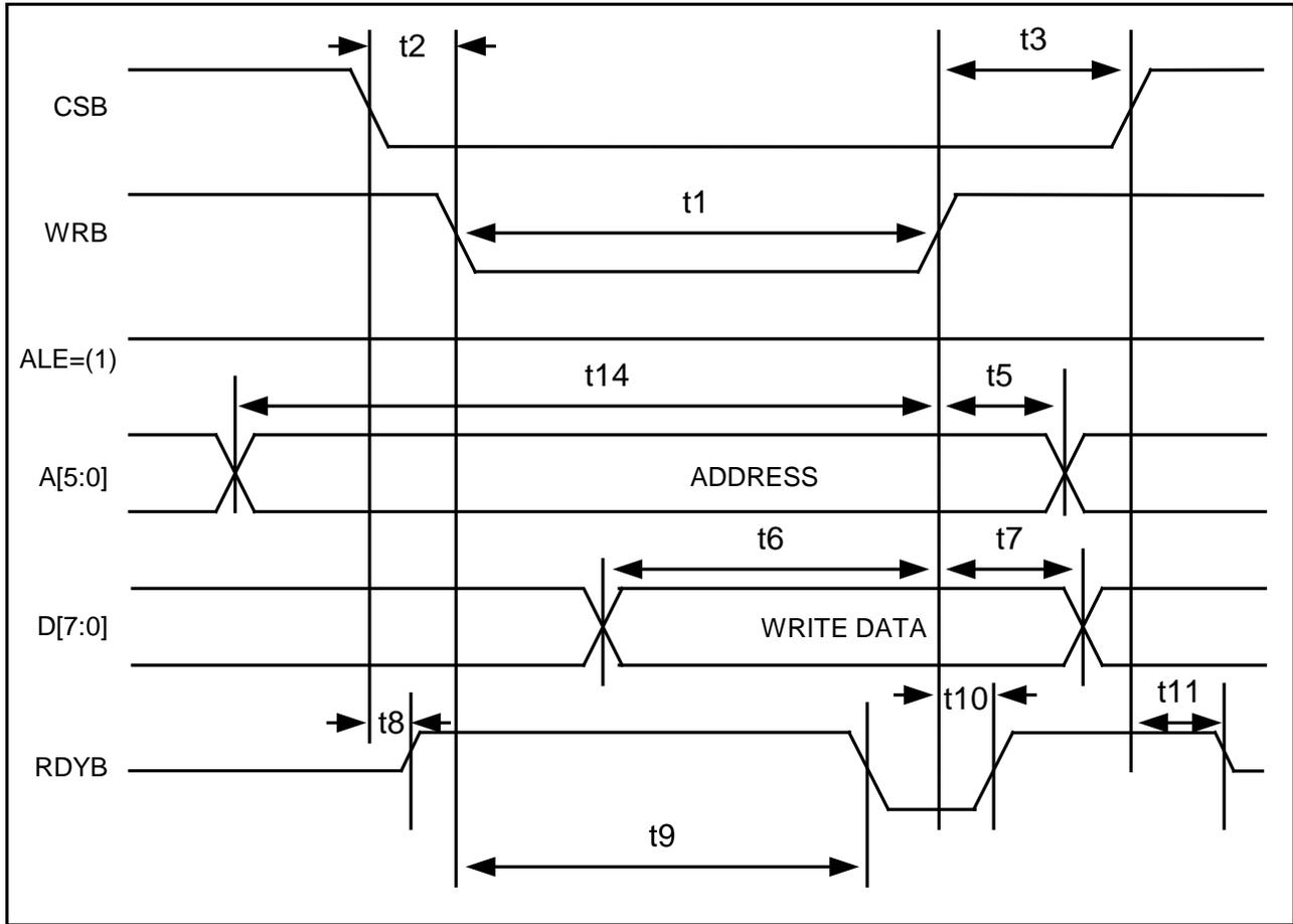
Figure 9-4. Intel Mux Write Cycle
