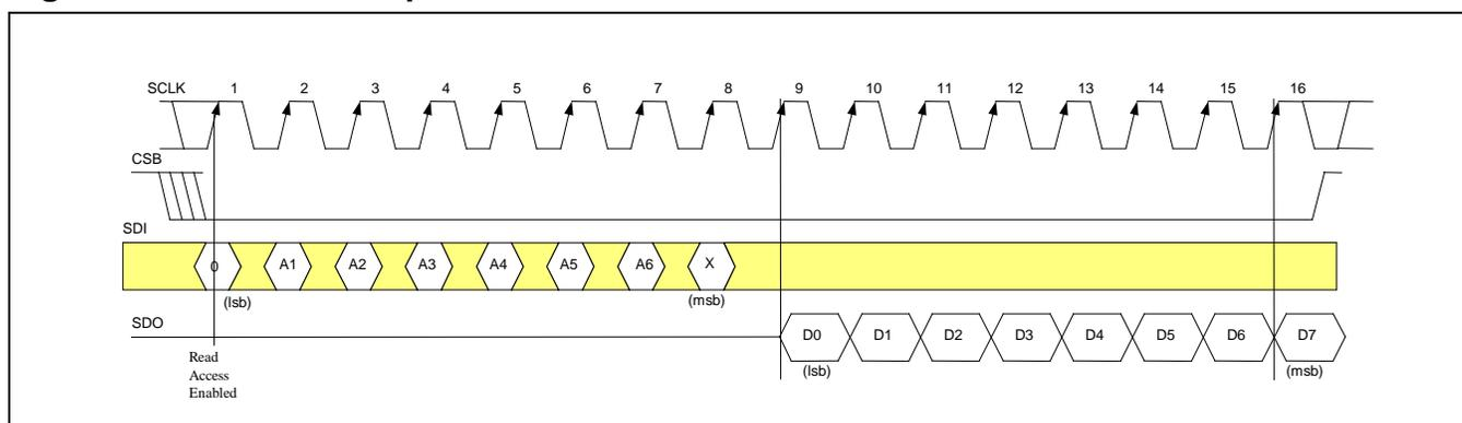
**Figure 5-3. Serial Port Operation for Read Access with CLKE = 1**
