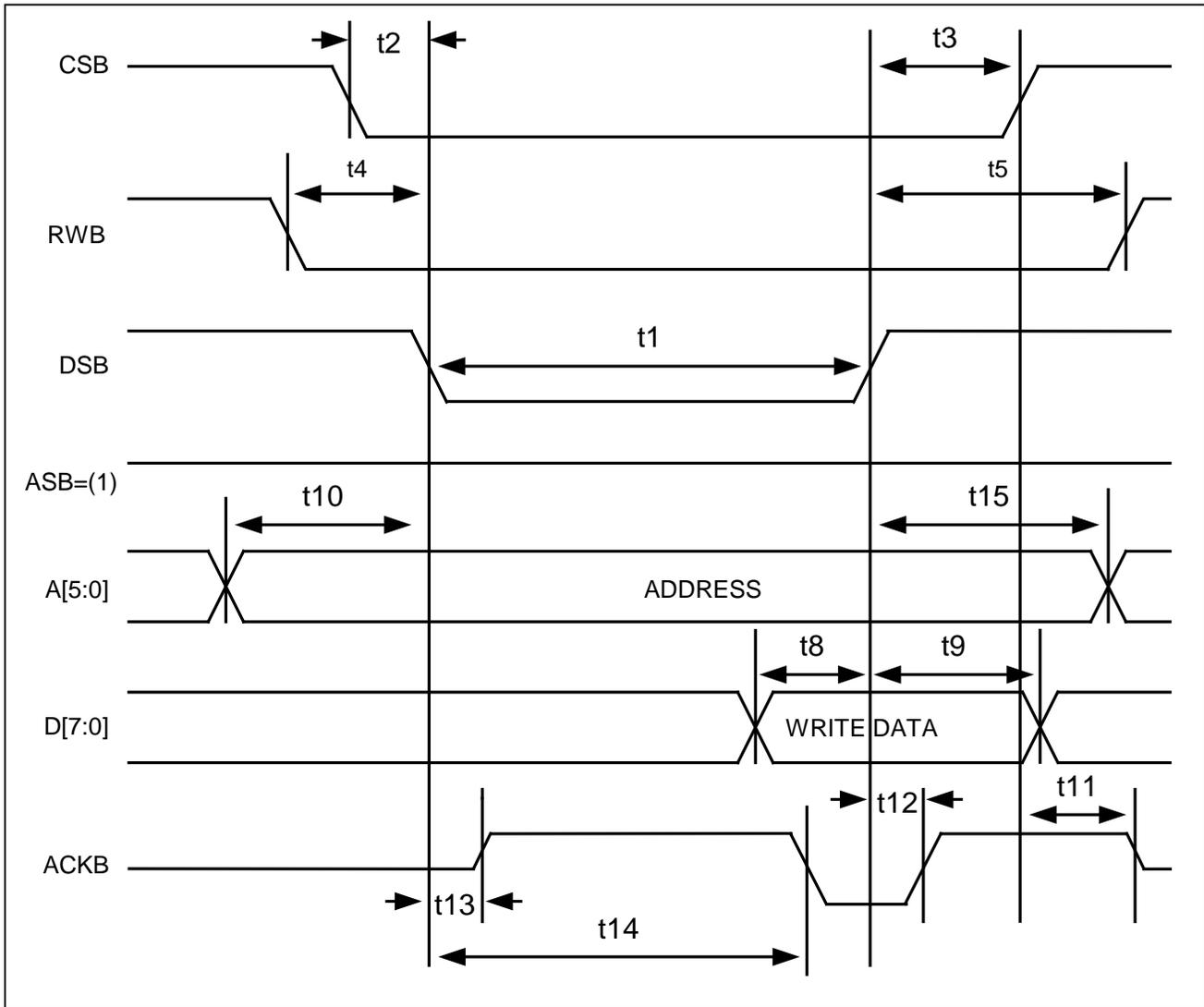
**Figure 9-8. Motorola Mux Write Cycle**
