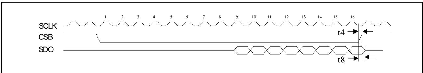
**Figure 9-11. Serial Bus Timing Read Operation with CLKE = 1**
