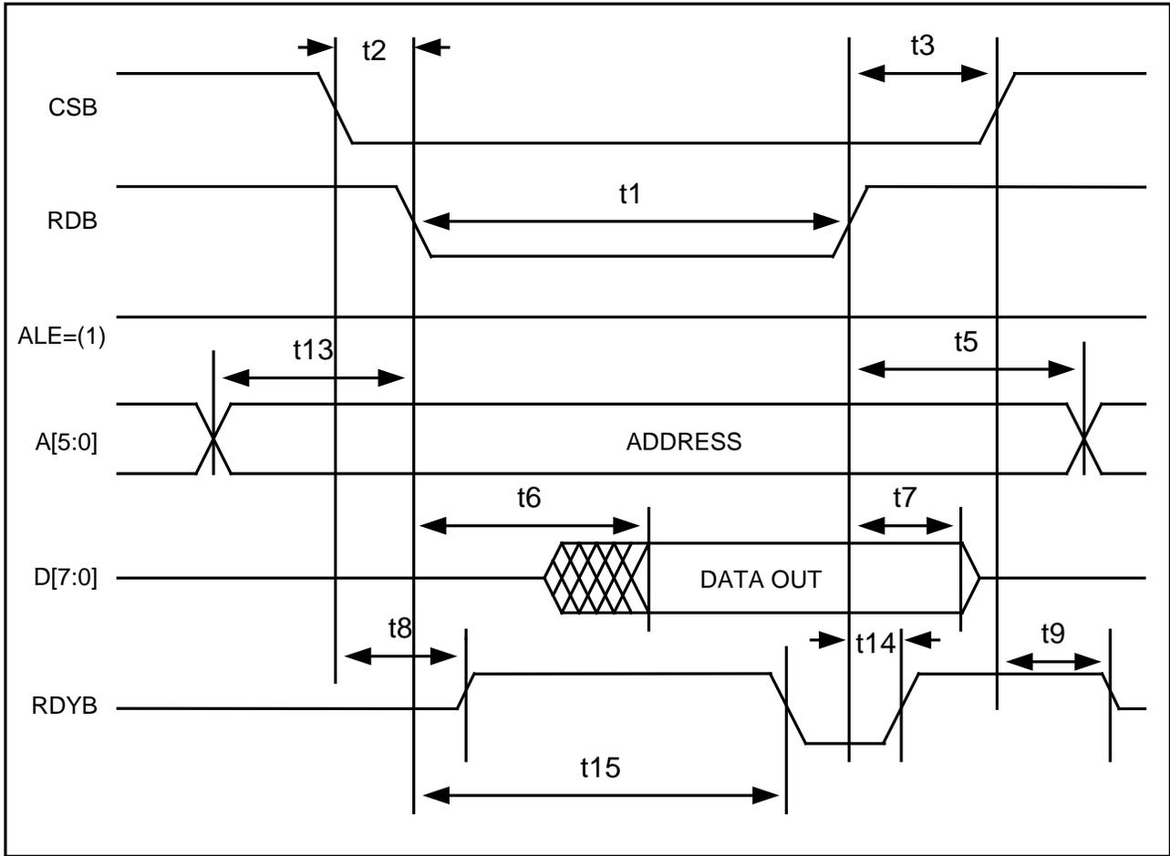
Figure 9-2. Intel Mux Read Cycle
