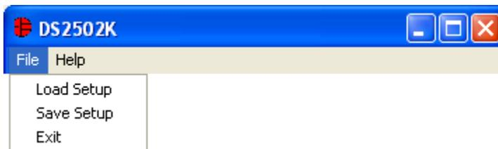
The File Menu allows the user to save or load all of the data in the text boxes on the Memory Tab. Selecting the Load Setup does not write the DS2502, but rather it loads the values into the text boxes. The user must still click the Write button in order to write the device.
