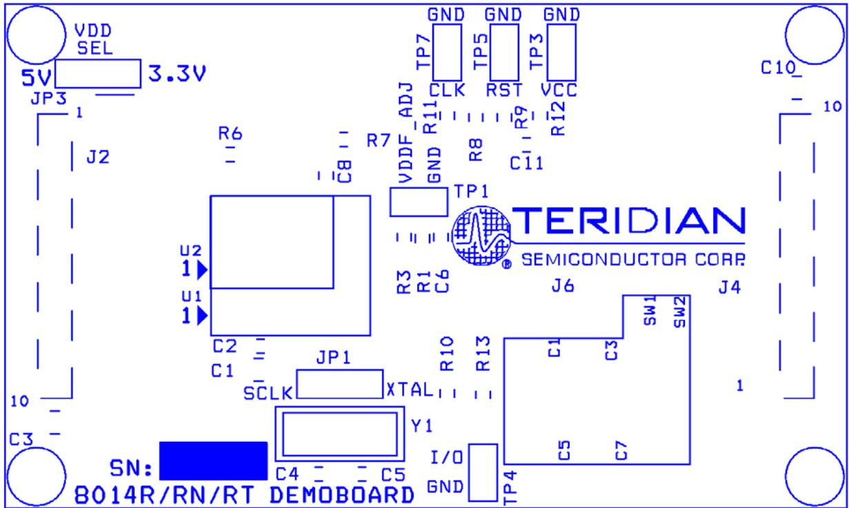
Figure 6: TERIDIAN 73S8014R/RN/RT 20SO Demo Board: Bottom View
