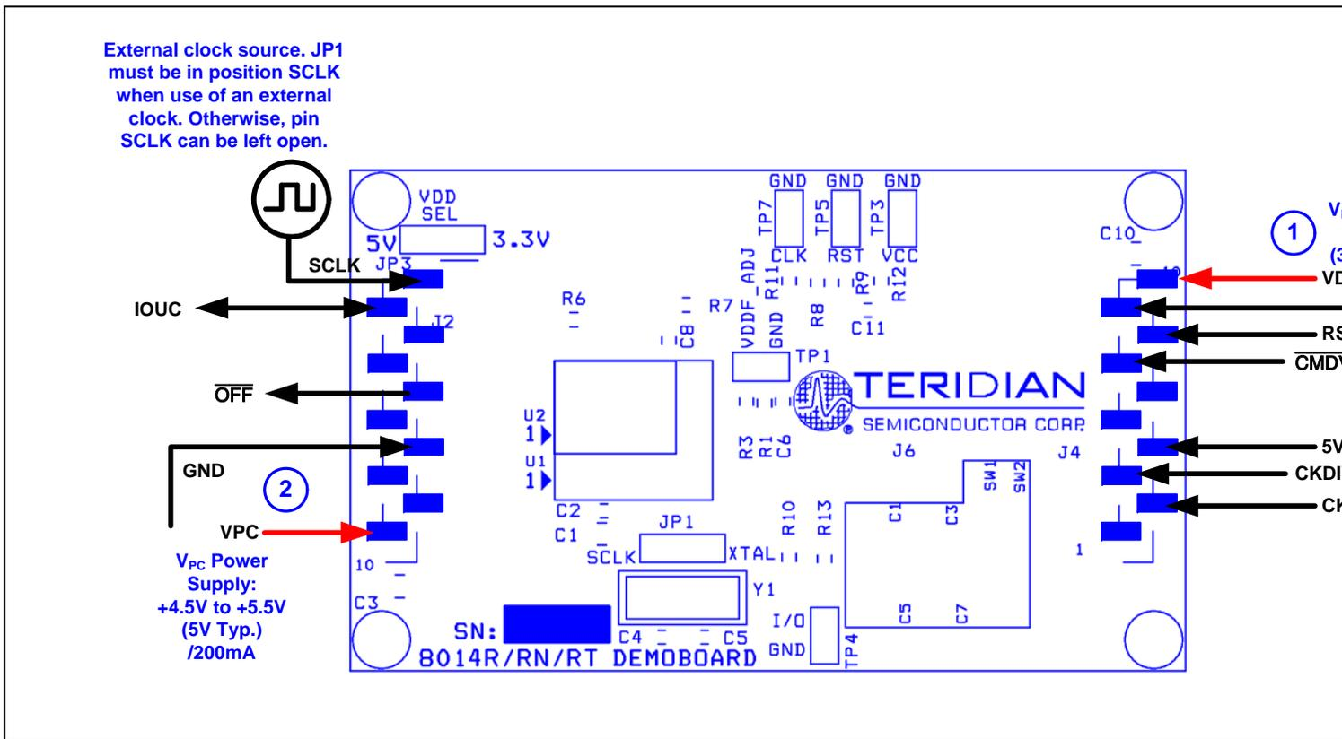
Figure 2: 73S8014R/RN/RT Demo Board: Basic Connections
