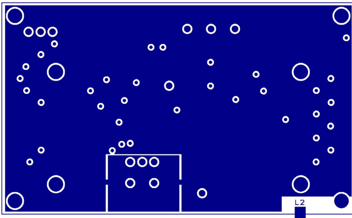
Figure 9: TERIDIAN 73S8014R/RN/RT 20SO Demo Board: Middle Layer 2, Supply Plane.
