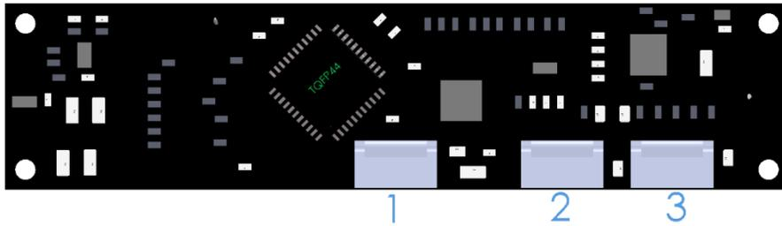
Figure 2: LK162A-4T Standard and USB Module Header Locations
