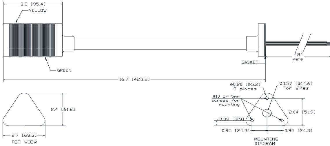
**LED OPERATION:** CONNECT STACK COLOR WIRE TO POWER AND BROWN WIRE TO POWER.
