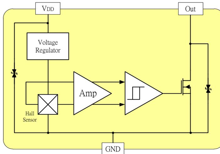
**Note:** Static sensitive device; please observe ESD precautions. Reverse  $V_{DD}$  protection is not included. For reverse voltage protection, a 100  $\Omega$  resistor in series with  $V_{DD}$  is recommended.
