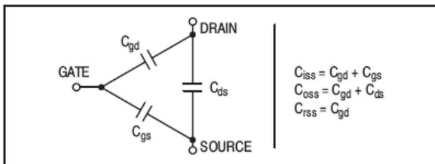
The  $C_{iss}$  given in the electrical characteristics table was measured using method 2 above. It should be noted that  $C_{iss}$ ,  $C_{oss}$ ,  $C_{rss}$  are measured at zero drain current and are provided for general information about the device. They are not RF design parameters and no attempt should be made to use them as such.
