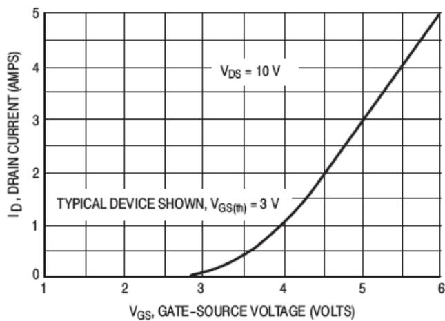
Figure 5. Drain Current versus Gate Voltage (Transfer Characteristics)
