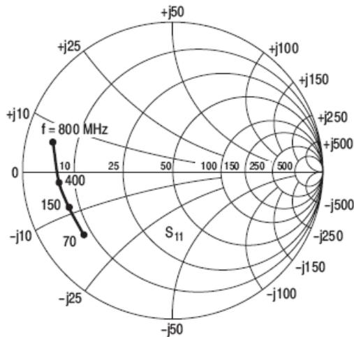
Figure 19.  $S_{11}$ , Input Reflection Coefficient versus Frequency
