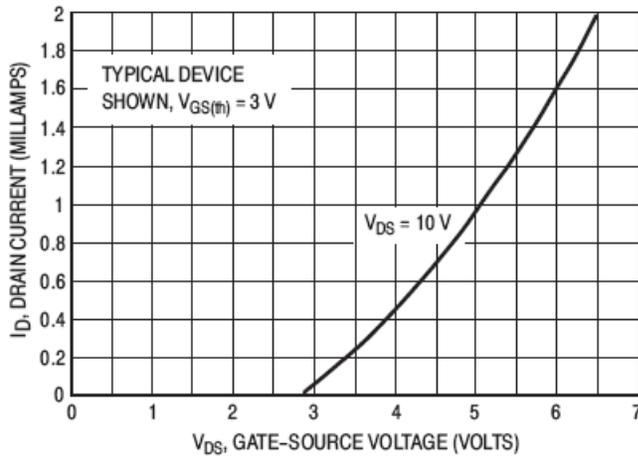
Figure 8. Drain Current versus Gate Voltage (Transfer Characteristics)\*
