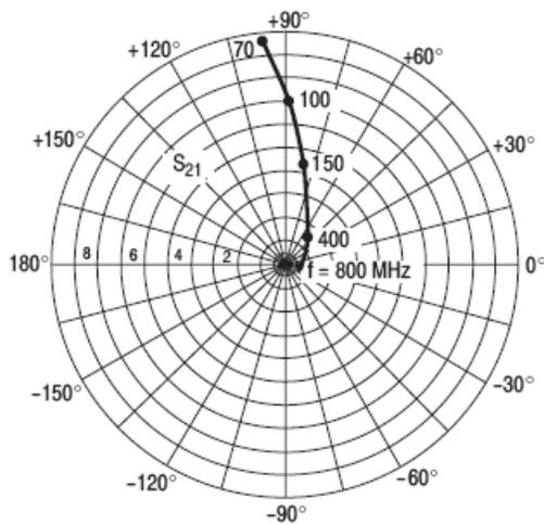
Figure 21.  $S_{21}$ , Forward Transmission Coefficient versus Frequency
