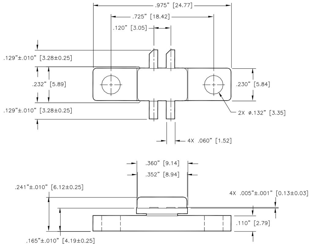
Unless otherwise noted, tolerances are inches  $\pm$ .005" [millimeters  $\pm$ 0.13mm]
