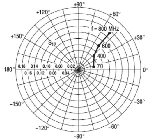
Figure 20.  $S_{12}$ , Reverse Transmission Coefficient versus Frequency
