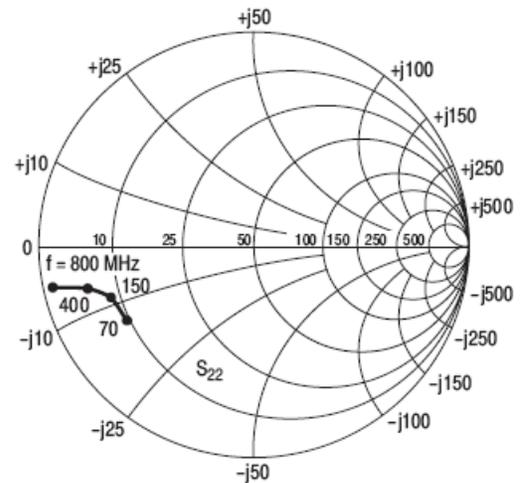
Figure 22.  $S_{22}$ , Output Reflection Coefficient versus Frequency
