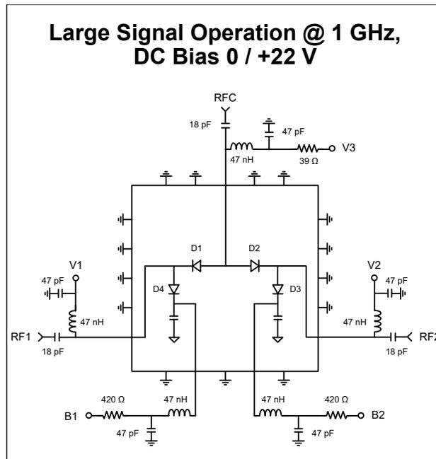
In order to safely operate at 100 W incident power, the values of the reactive components that make up the bias decoupling networks and DC blocking must be rated appropriately. Proper heat sinking is essential to safe operation under high incident power.
