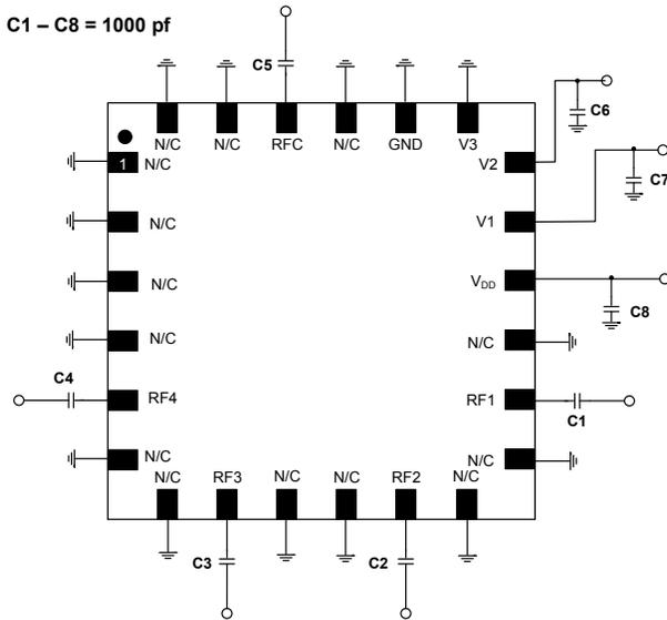
13. Configuration shown is for optional 2 control operation which does not include an All-Off condition. V3 pin must be connected to Ground externally as shown.
