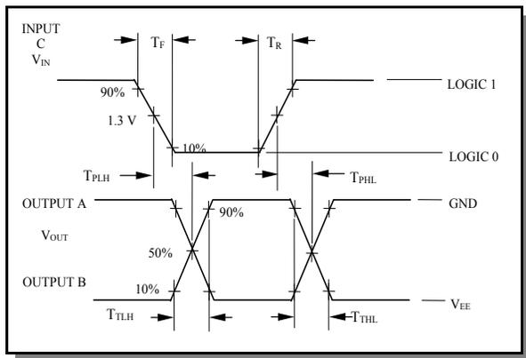
Note: See Switching Wave Forms for the definition of the switching terms. Supplies must be by-passed with .01  $\mu\text{F}$  Capacitors.
