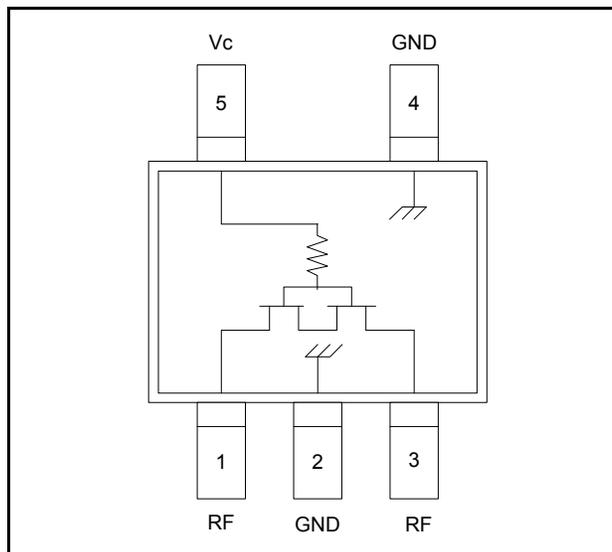
3.  $V_C = -3\text{ V to }0\text{ V @ }25\text{ }\mu\text{A maximum.}$
