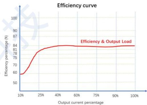
Figure 5: Efficiency VS Output Load (Nominal Voltage Input)
