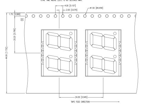
\*UNLESS OTHERWISE SPECIFIED TOLERANCES PER DECIMAL PRECISION ARE: X=±1 (±0.039), X.X=±0.5 (±0.020), X.XX=±0.25 (±0.010), X.XXX=±0.127 (±0.005). LEAD SIZE=±0.05 (±0.002), LEAD LENGTH=±0.75 (±0.030). MIN=  $^{+DECIMAL}_{-0.00}$  PRECISION MAX.=  $^{+0.00}_{-DECIMAL}$  PRECISION  $^{+0.00}_{-$
