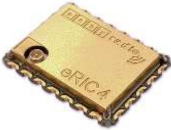
The easy Radio Intelligent Controller (eRIC) radio transceiver module is based on the Texas Instruments CC430F5137 System-on-Chip device to provide an intelligent radio sub-system that combines a high performance RF transceiver, RF band pass filters (BPF), an MSP430 microcontroller, 32Kb flash memory, non-volatile flash storage, temperature sensor, and a low drop voltage regulator. The device operates on the International licence exempt Industrial, Scientific and Medical (ISM) radio bands.
