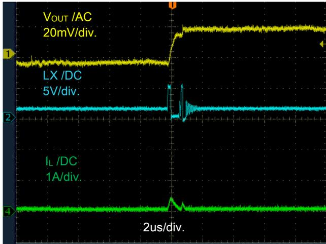
$V_{IN}=5V, V_{OUT}=1.2V, I_{OUT}=1A$
