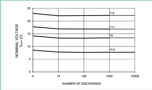
**Fig. 6 1206 Size Pulse Rating for Long Duration Surges (Any Single Section)**
