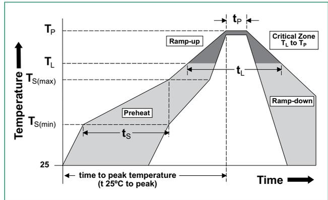
**Soldering Parameters - Wave Soldering (Thru-Hole Devices)**
