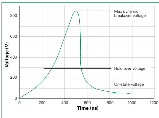
**Note:** Tested per 1kV/µs waveform
