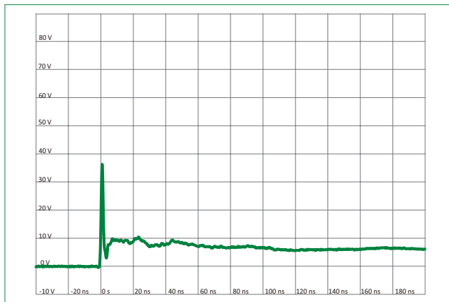
IEC 61000-4-2 +8 kV Contact ESD Clamping Voltage
