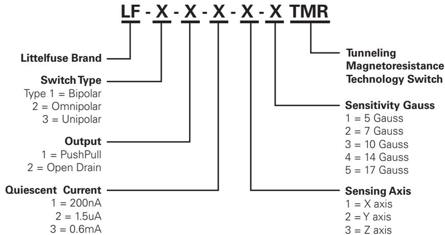
Example: LF11115 is Bipolar, Push Pull, 200 nA, X axis, 17 Gauss.
