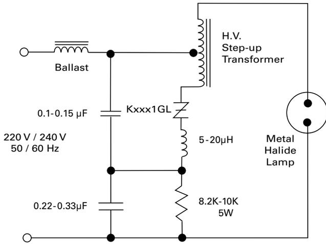
Note: With proper component selection, this circuit will produce three pulses for ignition of metal halide lamp that requires a minimum of three pulses at 5kV magnitude and >1µSec duration each at a minimum repetition rate of 3.3kHz.
