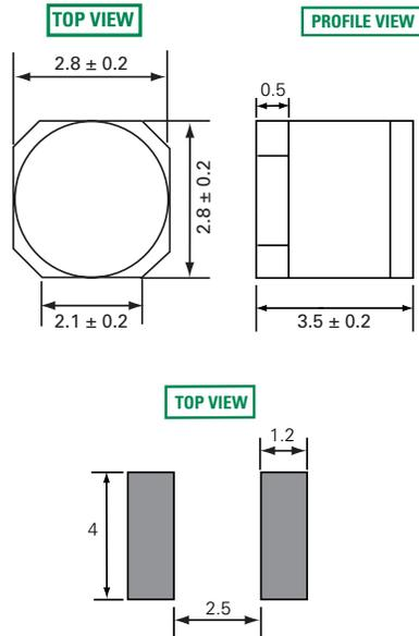
Recommended Soldering Pad Layout
