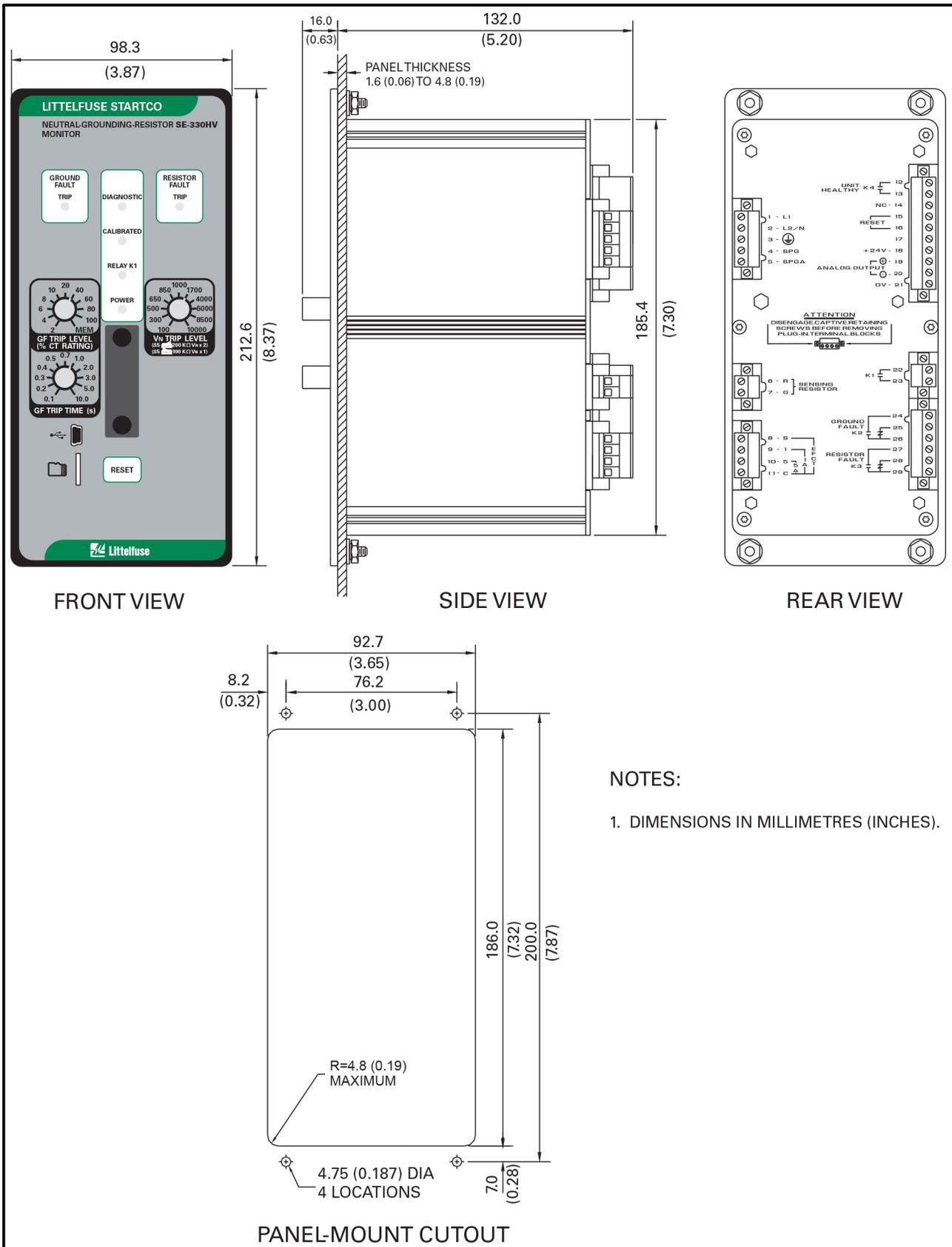
FIGURE 4. SE-330HV Outline and Panel-Mounting Details.
