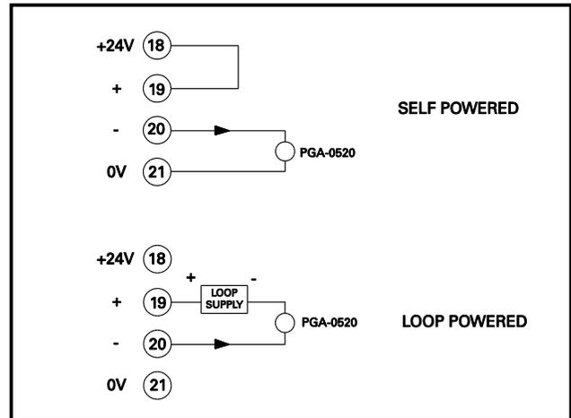
FIGURE 2. Analog-Output Connections.
