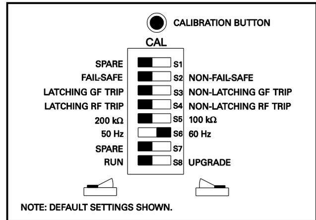
FIGURE 1. Configuration Switches.
