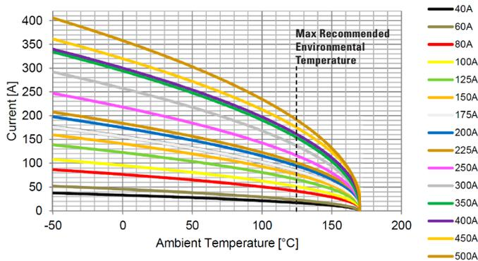
Derating curves may change depending on the final condition of the application (terminals characteristics, wire size etc.).
