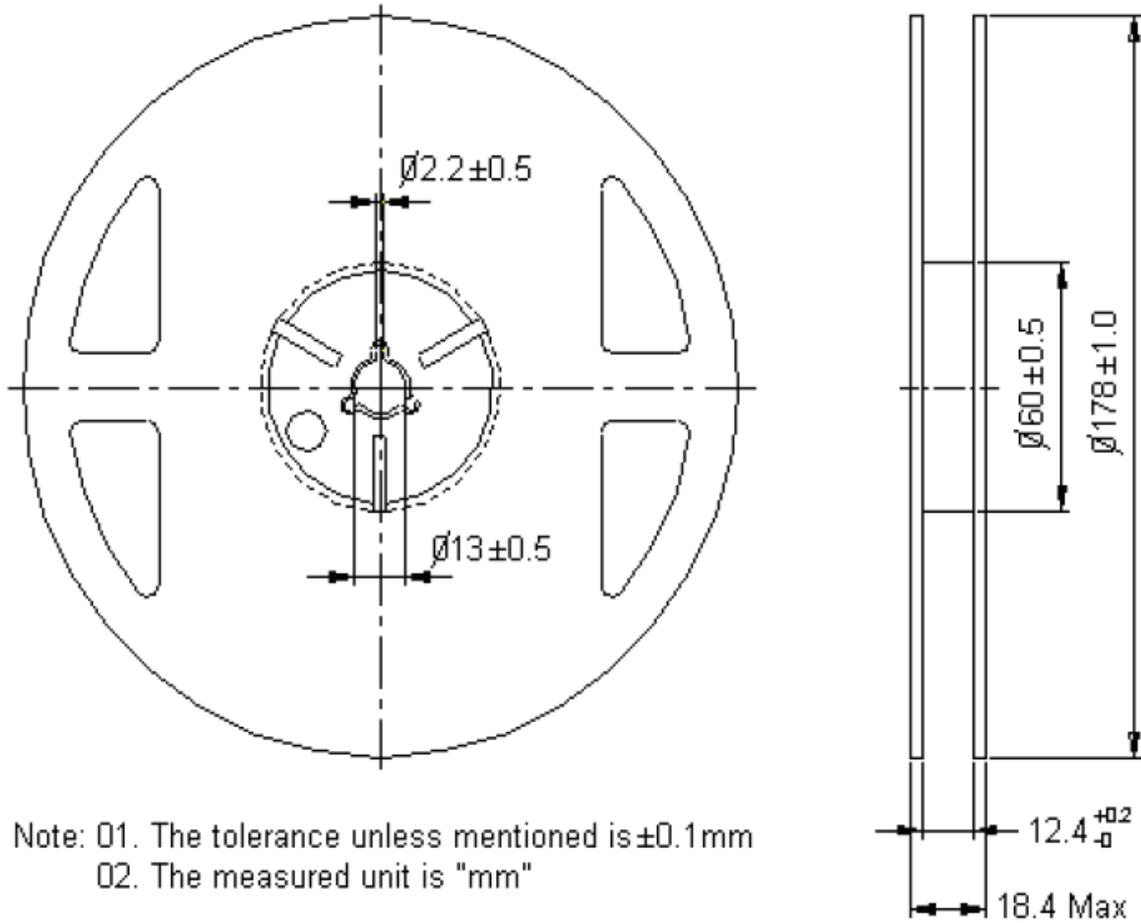
Note: 01. The tolerance unless mentioned is  $\pm 0.1$  mm
