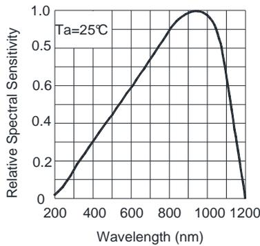
FIG.1 SPECTRAL SENSITIVITY
