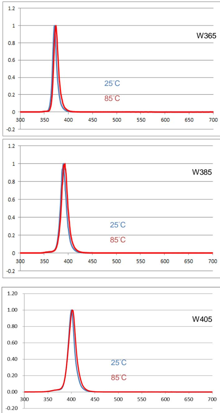
Fig 2. Relative Spectral Distribution at T<sub>j</sub> = 25°C & 85°C
