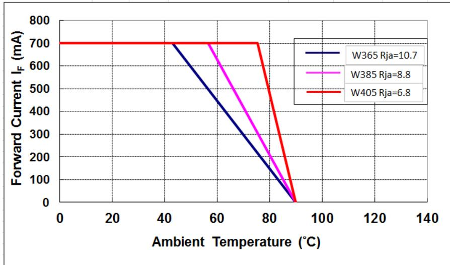
Fig 5. Forward Current Degrading Curve of LTPL-C034UVHXXX
