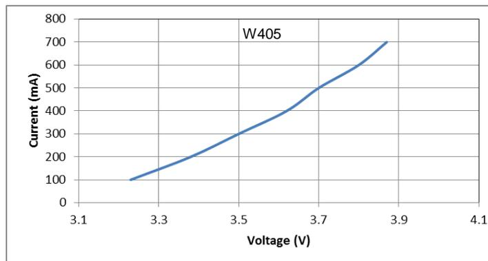
Fig 4. Forward Current vs. Forward Voltage of LTPL-C034UVHXXX
