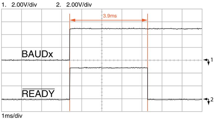
Figure 19: NT Series Transceiver Baud Band Change Time
