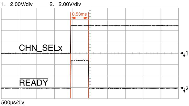
Figure 18: NT Series Transceiver Channel Change Time
