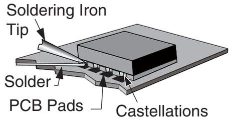
Figure 35: Soldering Technique
