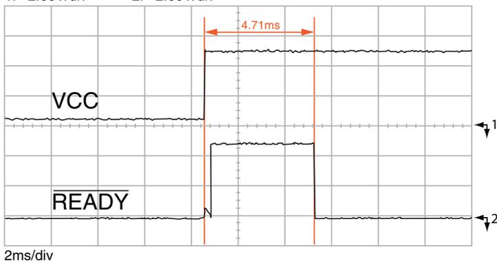
Figure 13: NT Series Transceiver Turn-On Time from VCC
