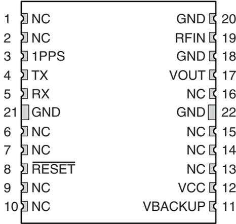
Figure 5: FM Series GPS Receiver Pinout (Top View)
