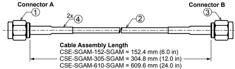
Figure 1. Product Dimensions for the CSE-SGAM-ccc-SGAM Cable Assembly
