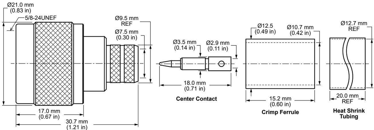
Figure 1. Product Dimensions for the CONN007-1-W Connector
