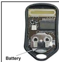
Figure 4: Battery Access
