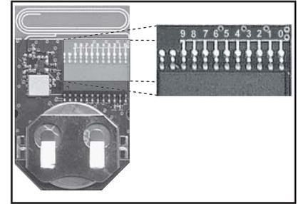
Figure 2: DIP Switch Assignments
