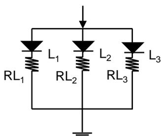
Fig.1 Recommended Circuit in Parallel Mode
