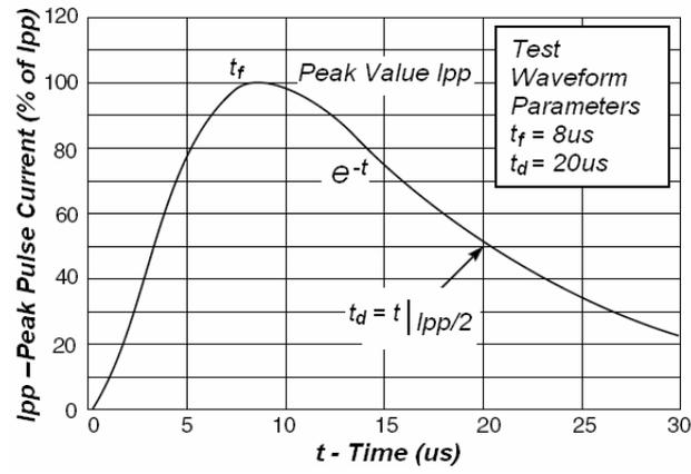
Fig3. Pulse Waveform
